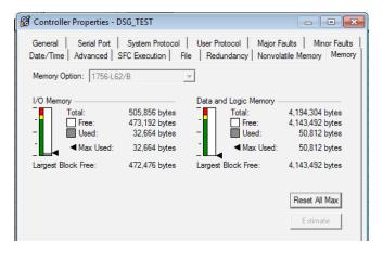
FIG.2. PLC CPU memory performance when *local* PLC chassis is connected with *remote* #1 and *remote* #2 PLC chassis via Controlnet network.
