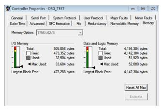
FIG. 4. PLC CPU memory performance when *local* and *remote #1* are connected via Controlnet network and *local* and *remote #2* PLC chassis via Ethernet modules.
