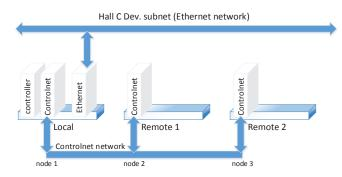
FIG. 1. Setup with only Controlnet modules
